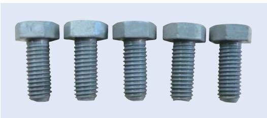
Combined cycle corrosion test (JASO M609-91)
