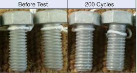
Combined cycle test(JASO M609-91)(Electrolytic corrosion test)(Stainless steel bolts tighten into the aluminium board)
